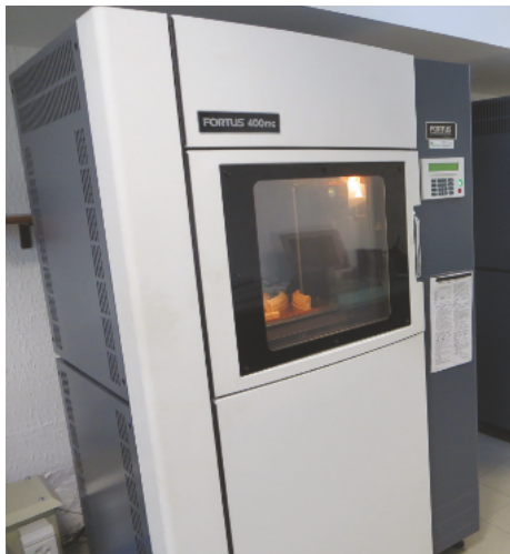
Stratasys' Fortus 400mc 3D production system produces parts that include Nolders - an aerodynamic profile installed under vehicle bumpers
